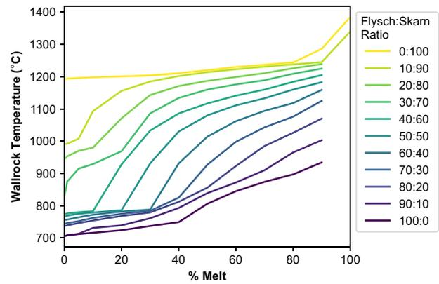
**Fig. 6.** The physical state of various wallrock compositions (plotted by mixing ratios of flysch:skarn) at temperatures from their solidus (0% melt) to liquidus (100% melt) determined by rhyolite-MELTS. Solutions for liquids are not shown where rhyolite-MELTS did not converge on one. Note the broad range in wallrock solidi from flysch (100:0, 706 °C) to skarn (0:100, 1193 °C) and that the addition of just 10% of flysch to skarn (i.e. 10:90) lowers the wallrock solidus by over 200 °C.
