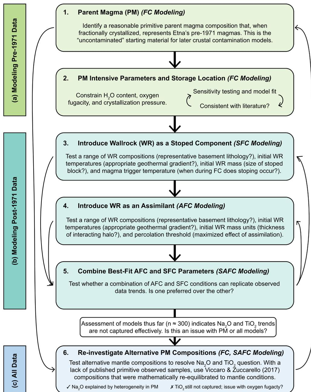
**Fig. 3.** Flowchart illustrating a general roadmap of the MCS modeling process, which was initially broken into two steps with goals of modeling (a) pre-1971 data and (b) post-1971 data. Due to undesirable fit of Na<sub>2</sub>O and TiO<sub>2</sub> (wt.%) in all models, (c) alternative PM compositions were re-investigated.
